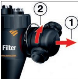
3. Push the inlet/outlet port back towards the body of the unit to prevent further rotation.
